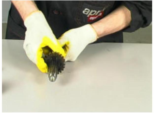
**4.1.3. TRANSMISSION SHAFT DISASSEMBLY**
