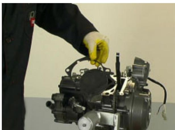
**NOTE** Before removing the gudgeon pin circlip, block off the casing opening with a clean cloth to prevent the circlip from falling inside the crankcases.
