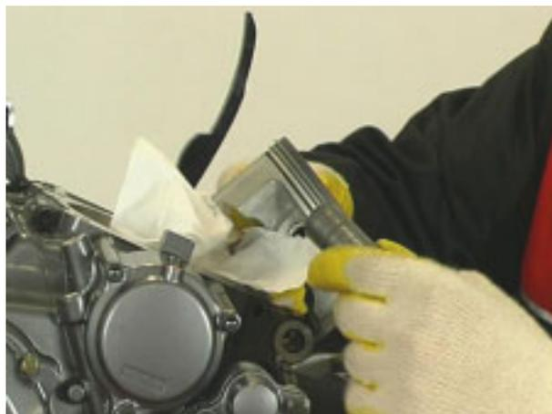
**NOTE** Before fitting the gudgeon pin circlip, block off the casing opening with a clean cloth to prevent it from falling inside.
